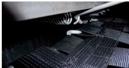
Hinging or unhinging the steel springs with the mounting tool
