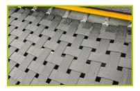
**7- The trampoline surface** is made up of a series of straps, reinforced with steel cables; the straps are joined to the frame by steel springs.
