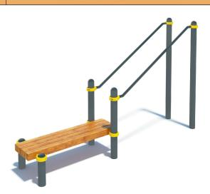
The complex consists of six backup columns at the height of: 2000 mm- 2 pieces, 1100 mm- 2 pieces, 450 mm -2 pieces. The complex includes inclined parallel bars with bench. Inclined parallel bar height difference- 966mm, length 1790mm, diameter 42mm, height 1000mm. Crossbar length: 2 pieces- 500mm, diameter 34mm. All bars are fixed to backup columns by means of collars. Weight - 166.00 kg.
