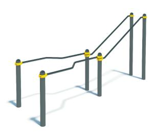
The complex consists of six backup columns at the height of: 2000 mm- 2 pieces, 1100 mm- 4 pieces. The complex includes multi-width parallel bars and inclined parallel bars. Distance between multi-width parallel bars- 1208mm at one end and 608mm- at another end, lenght of bars- 1790mm, bar diameter 42mm, height - 1100mm. Inclined parallel bar height difference- 966mm, lenght 1790mm, diameter 42mm, height -1000mm. All bars are fixed to backup columns by means of collars. Weight - 150.20 kg.
