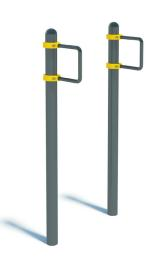
The complex consists of two backup columns at the height of 2000 mm. U-type parallel multi-hold bars are fixed to backup columns at the height 1800mm by means of collars. Bar diameter 34 mm, size- 300mm x 300mm. Weight - 59.20 kg.
