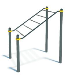
The complex consists of four backup columns at the height of: 2600 mm -2 pieces, 2000 mm - 2 pieces. Monkey bar is fixed to backup columns at the height 1500mm and 2466mm by means of collars. The distance between bars is 400 mm, width 1308 mm, height difference 966,3mm. Total length of inclined monkey bar- 1790mm. Weight - 153.60 kg.
