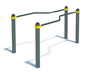
The complex consists of four backup columns at the height of: 1100 mm. Parallel bars are fixed to backup columns at the height of 1100 mm by means of collars. Bar diameter 42 mm, total length 1790mm. Weight - 79.80 kg.
