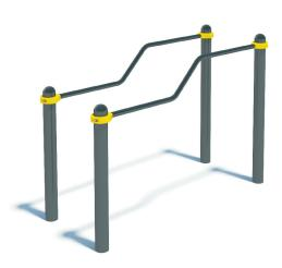
The complex consists of four backup columns at the height of: 1400 mm -2 pieces, 1100 mm-2 pieces. Parallel bars are fixed to backup columns at the height 1100mm and 1400mm by means of collars. The distance between bars is 608 mm, total lenght 1790mm, bar diameter 42 mm. Weight - 88.00 kg.
