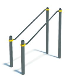
The complex consists of four backup columns at the height of: 2000 mm -2 pieces, 1100 mm-2 pieces. Parallel bars are fixed to the backup columns at the height of 1000 mm and 1966mm by means of collars. The distance between bars 608mm, bar diameter 42 mm, total bar length 1790mm. Weight - 101.20 kg.
