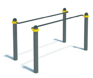
The complex consists of four backup columns at the height of 1100 mm. Parallel bars are fixed at height 1100 mm by means of collars. Parallel bar diameter 34mm, total length of bars- 1932mm. Distance between parallel bar inner surface - 550mm. Weight - 77.60 kg.
