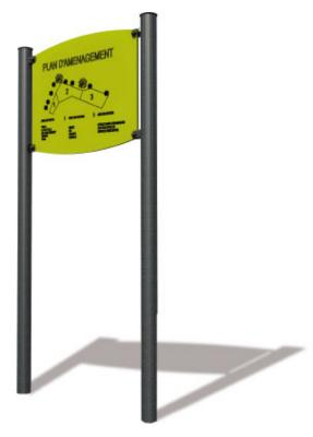
manufactured from Panels 13mm thick compact-Black powdercoated, galvanised steel post 102mm diameter, thickness 2mm- Post protected by an aluminium cap - Panel personalised by engraving- stainless steel fixings
