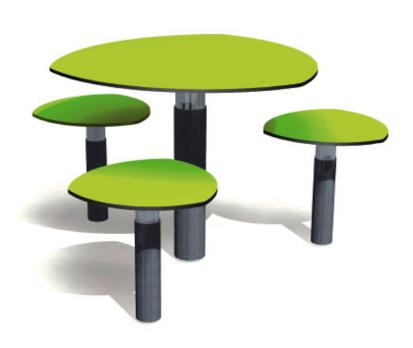
Table and seat tops manufactured from 13mm thick compact - Black polyester powdercoated steel posts for table and stools. Table: diameter 125mm, thickness 2.5mm Stool: diameter 102mm, thickness 2mm. Stainless steel fixings protected by ployamide anti-vandal caps
