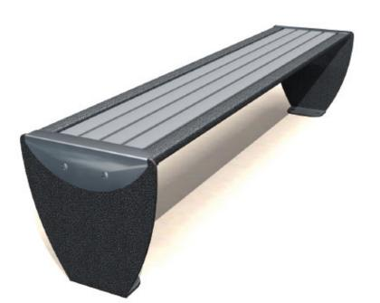
Seat comprises 2 painted steel slats 50x25x2,5 mm, and 4 pultruted polyester slats (polyester composite/fibre glass) 58x25x3 mm, RAL 7004. Black polyester powdercoated steel base, thickness 8mm - Stainless steel brackets and fixings - Fixing on to a concrete block
