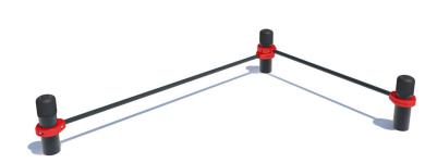
The construction consists of 3 vertical columns\* and two crossbars\*\* placed on the following heights: 200 mm- 1pcs.,250mm- 2 pcs. and 300 mm- 2 pcs. from the rubber foundation. Crossbar fittings are put into effect with collars\*\*\*. The length of crossbars is 1200 mm- 1pcs., 1700mm- 1pcs.. The height of columns is 400 mm. Weight - 77.5 kg
