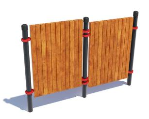
The construction consists of 3 vertical columns\* and two walls made from wooden beams, which are mounted on crossbars\*\* on the following heights: 400mm/1750mm, wall height 1900mm and 500mm/1850mm, wall height 2000mm from the rubber foundation. Wooden beam lengths are 1650mm. Crossbar fittings are put into effect with collars\*\*\*. The length of all crossbars is 1200 mm. The height of columns is 2000mm. Weight - 326.9 kg
