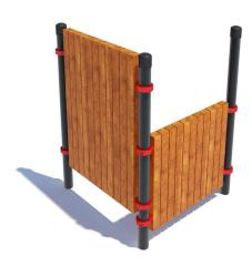
The construction consists of 3 vertical columns\* and two different height walls made from wooden beams, which are mounted on crossbars\*\* on the following heights: 300mm/1050mm, wall height 1200mm and 500mm/1850mm, wall height 2000mm from the rubber foundation. Wooden beam lengths are 1050mm for the low wall and 1650mm for the high wall. Crossbar fittings are put into effect with collars\*\*\*. The length of all crossbars is 1200 mm. The height of columns is 2000mm. Weight - 284.9 kg
