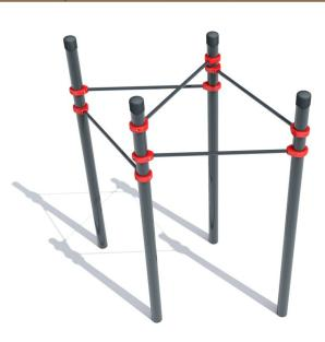
The complex consists of four vertical columns at the height of 2600 mm, 5 crossbars for pull-ups at the height of 2400 mm, 2300 mm, 2100 mm, 1900 mm. The length of crossbars is 1200 mm. Metallic construction of the pull-up bar is fixed with collars to the vertical columns. Weight 153 kg
