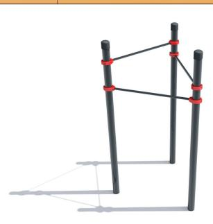
The complex consists from three vertical columns at the height of 2600 mm. Three crossbars for pull-ups. Crossbars are placed at the height of 2300 mm, 2100 mm, 1900 mm. The length of crossbars is 1200 mm. Metallic construction of pull-up bar is strengthened by means of collars to the vertical collumns. Weight 111 kg
