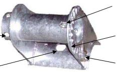
Cable clamp on the drum to fixing the ropes
